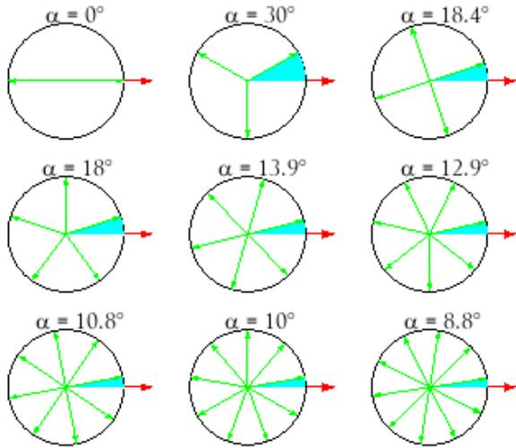
Figure 12. Optimized jettisoning direction regards to the orbital velocity (in red) and number of simultaneous ejections
