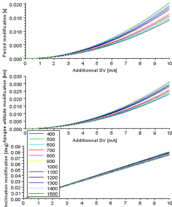
Figure 6. Impact on orbital period and apogee altitude and inclination of a  $\Delta V$  along W
