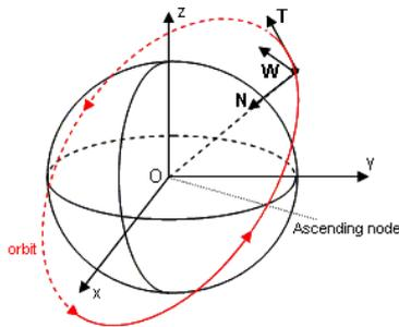
Figure 4. Local Orbital Frame Definition
