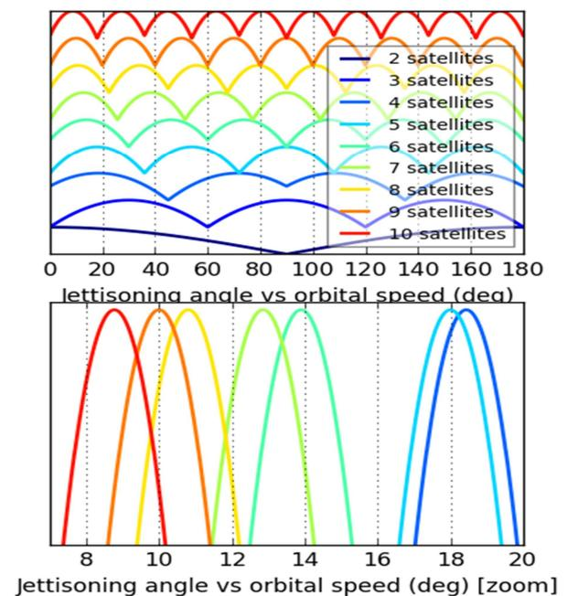
Figure 11. Optimization of the jettisoning angle (counted from the orbital velocity) and depending on number of simultaneously injected satellites
