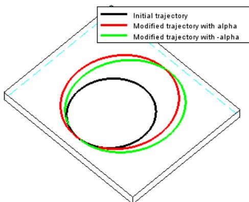
Figure 10. Orbit modification induced by a jettisoning as represented in Figure 9.1 of the composite (same semi-major axis, different argument of perigee)
