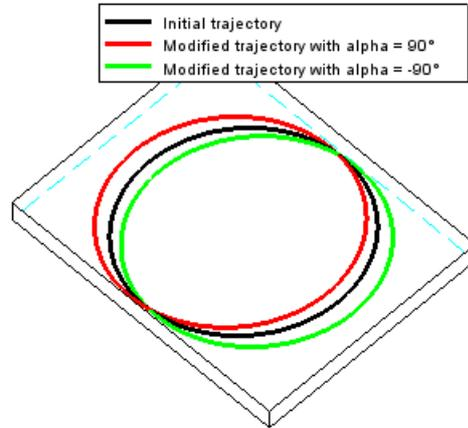
Figure 7. Obtained orbits after two jettisoning realized along  $\pm N$
