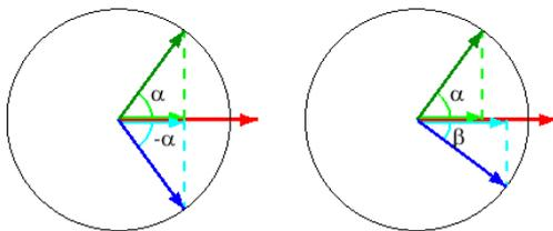
Figure 9.1 and 9.2 Projections of jettisoning  $\Delta V$  (green & blue) on the orbital velocity (red)
