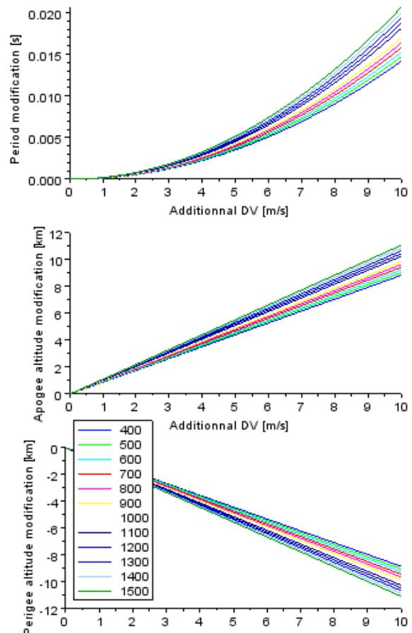
Figure 8. Impact on orbital period, apogee and perigee altitude of a  $\Delta V$  realized along  $\pm N$
