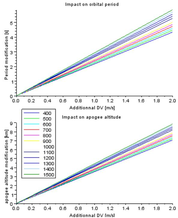
Figure 5. Impact on orbital period and apogee altitude of a  $\Delta V$  realized along T
