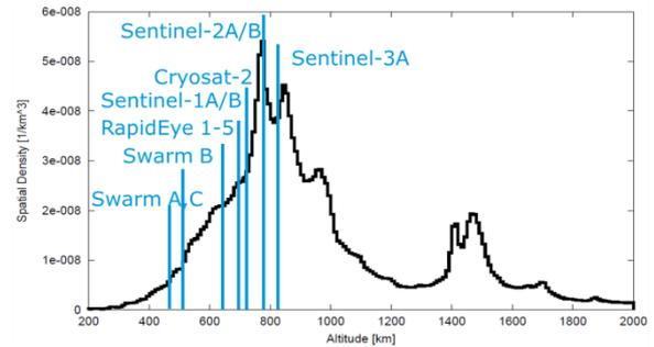
Figure 1. Missions in LEO currently covered by full collision avoidance support – operational altitudes and spatial density of objects > 10 cm (MASTER-2009)
