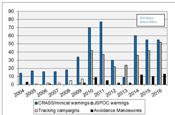
Figure 7. Collision avoidance statistics from ESA's SDO (end 2016).
