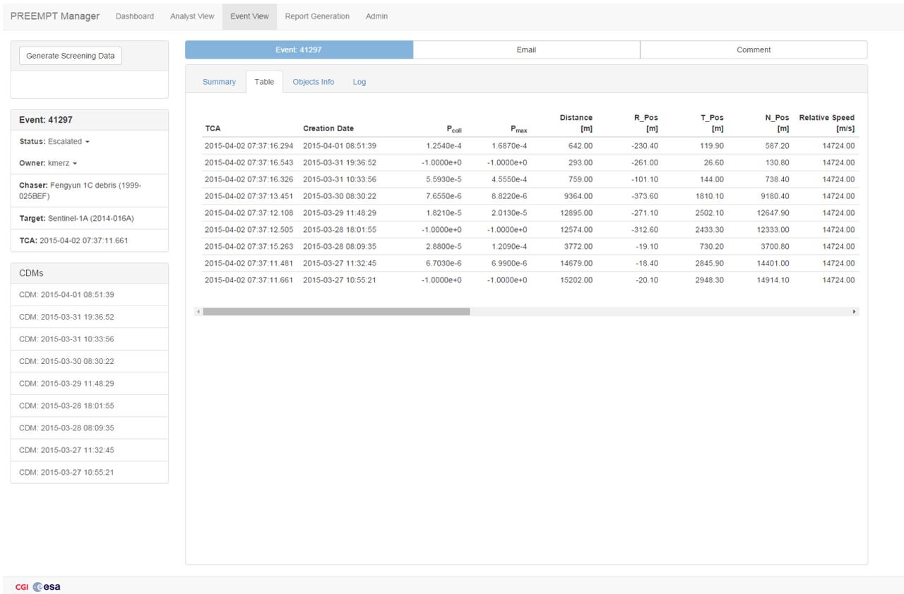
Figure 4. Screenshot showing the event view of the SDO's collision avoidance management tool SCARF.
