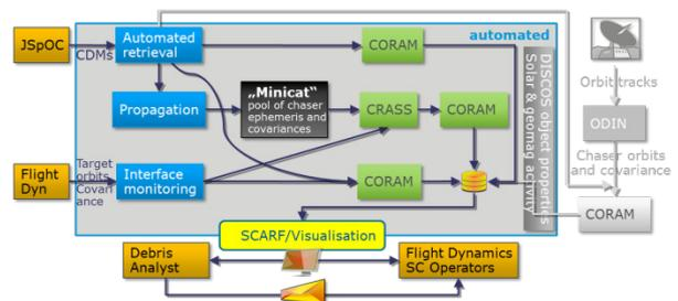
Figure 2. Extended operational collision avoidance process at ESA/ESOC with CDMs – current status
