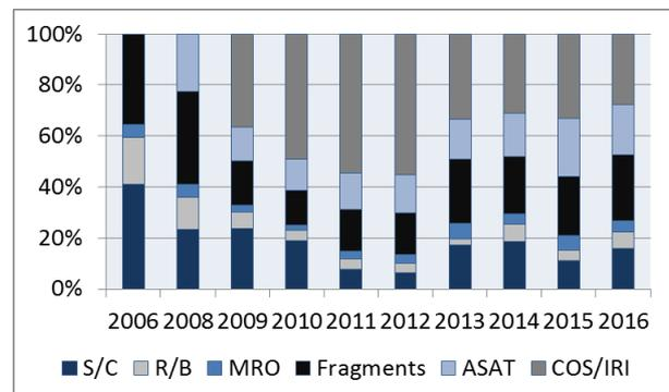
Figure 9. Classes of close approach objects sampling of the LEO environment - O/O vs. TLE orbits for all ESA missions.
