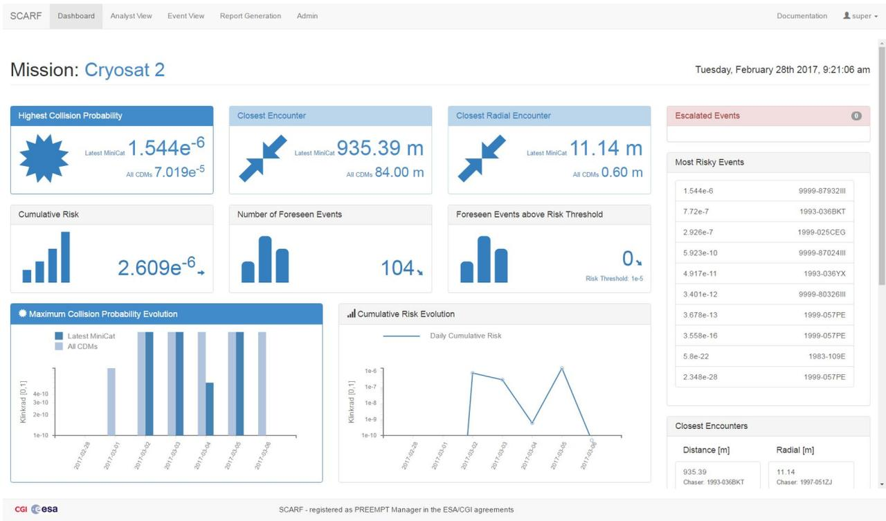
Figure 3. Screenshot showing the dashboard of the SDO's collision avoidance management tool SCARF.
