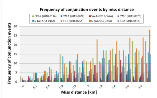
Figure 10. Frequency of conjunction events for Sentinel-1AB, -2A and -3A, Cryosat-2 and SWARM-A, -B and -C in 2016, grouped by miss distance (Sentinel-1B and -3A coverage starts June 2016), based on TLE screening
