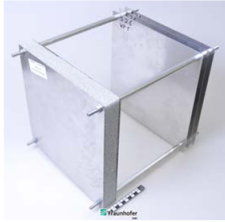
Figure 7: Sandwich panel target before impact testing (sample 2.6, experiment 5376).
