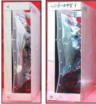
Figure 10. specimen after HVI test
