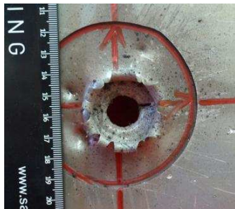
(a) Perforation in Al/Mg bumper for Shot A2-1#
