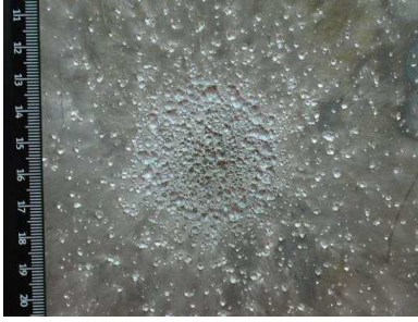
(b) Al/Mg shield ( V_p=4.486\text{km/s} , D_p=5.48\text{mm} )
