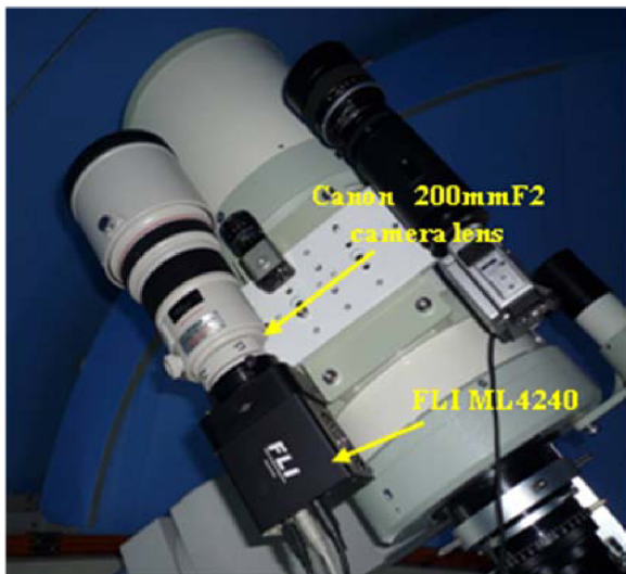
Figure 1. Optical observational unit which is composed of Canon 200mmF2 camera lens and FLI 2K2K back-illuminated CCD camera ML4240.
