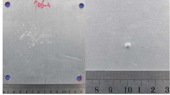
b. Front And Rear Of Third Wall Of “N” Configuration (V=3.00km/s)
