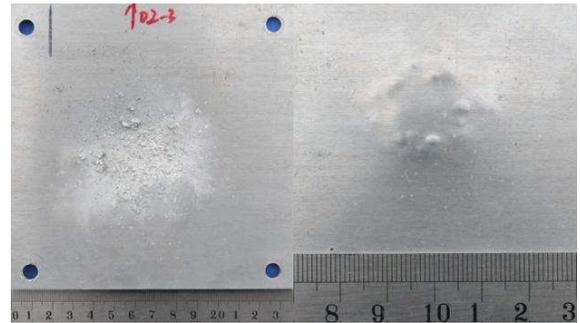
c. Front And Rear Of Third Wall Of Parallel Triple-wall Configuration (V=4.79km/s)
