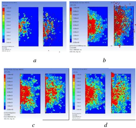
Figure 8. Comparisons Of Rear Plate Strain Of Simulation Results For Two Configurations(a.  $\Phi =4\text{mm}$ ,  $V=3\text{km/s}$ ,  $t=100\mu\text{s}$ ; b.  $\Phi =5\text{mm}$ ,  $V=4.8\text{km/s}$ ,  $t=100\mu\text{s}$ ; c.  $\Phi =5\text{mm}$ ,  $V=6\text{km/s}$ ,  $t=70\mu\text{s}$ ; d.  $\Phi =5\text{mm}$ ,  $V=7\text{km/s}$ ,  $t=60\mu\text{s}$ )
