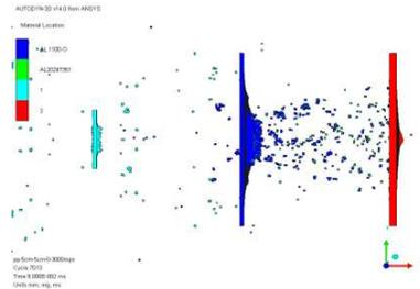
a. Parallel Triple-wall Configuration ( $\Phi=4.0\text{mm}$ ,  $V=3\text{km/s}$ ,  $t=80\mu\text{s}$ )
