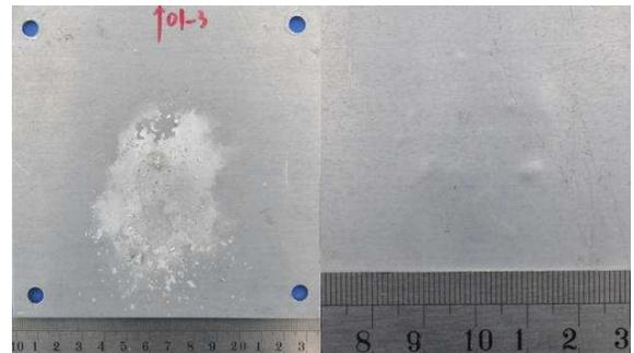
d. Front And Rear Of Third Wall Of “N” Configuration (V=4.85km/s)
