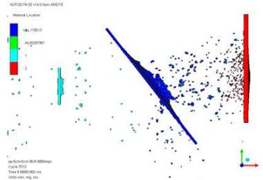
b. "N" Configuration ( $\Phi=4.0\text{mm}$ ,  $V=3\text{km/s}$ ,  $t=80\mu\text{s}$ )
