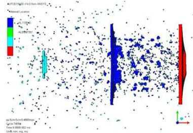
c. Parallel Triple-wall Configuration ( $\Phi=5.0\text{mm}$ ,  $V=4.8\text{km/s}$ ,  $t=80\mu\text{s}$ )
