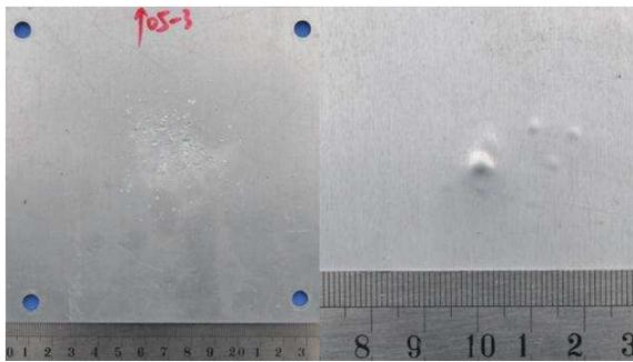
a. Front And Rear Of Third Wall Of Parallel Triple-wall Configuration (V=2.96km/s)
