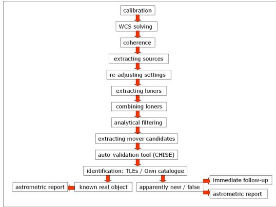
Figure 6. OAM processing software main steps
