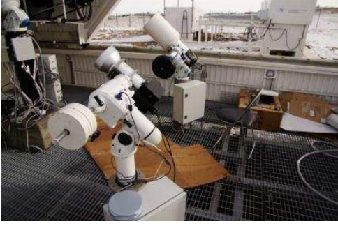
Figure 1. UN ORT optical camera, 15 sm. aperture, 11°x7° FOV (Kislovodsk, Tiraspol, Blagoveschensk, Kitab)
