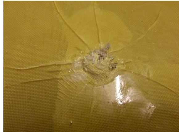
Figure 14. Bullets velocity of 1100 m/s at 4000 V of capacitors charging voltage.
