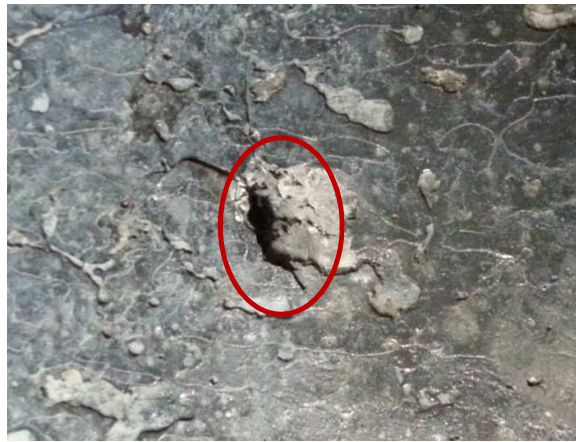
Figure 24. Damage of nanostructured Kevlar CFRP layered materials, zoom.
