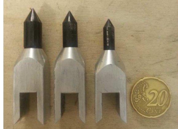
Figure 11. Bullets pictures: the armature is made of aluminium while the upper part of tungsten.
