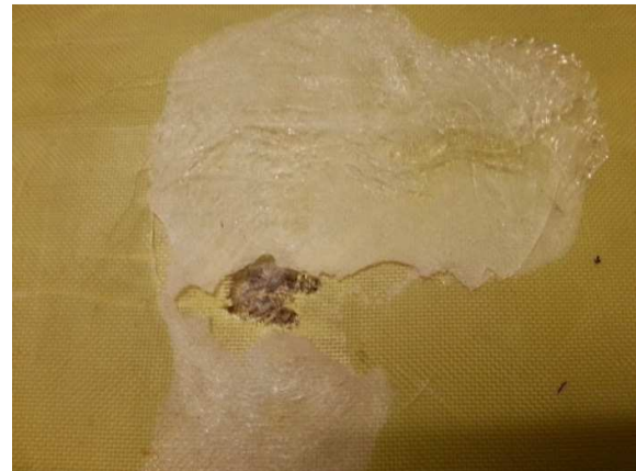
Figure 15. Damages of Kevlar based materials: sample front side (up), back side (down).
