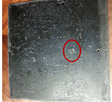
Figure 23. Damages of nanostructured Kevlar CFRP layered materials.
