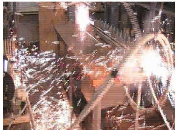
Figure 19. Railgun instant 4 of fire last 2ms.
