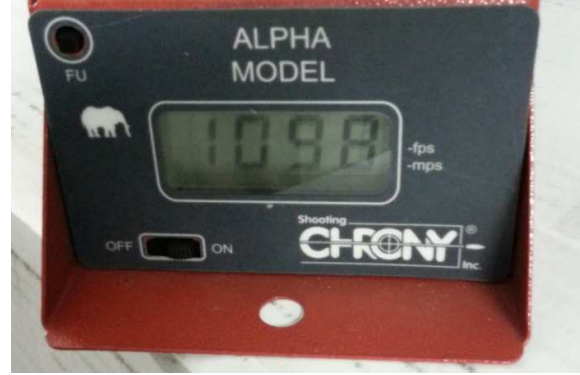
Figure 14. Bullets velocity of 1100 m/s at 4000 V of capacitors charging voltage.
