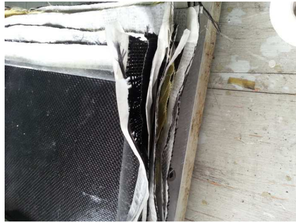
Figure 3. First kind of layered material. First layered CFRP+Kevlar structure before mechanical machining.
