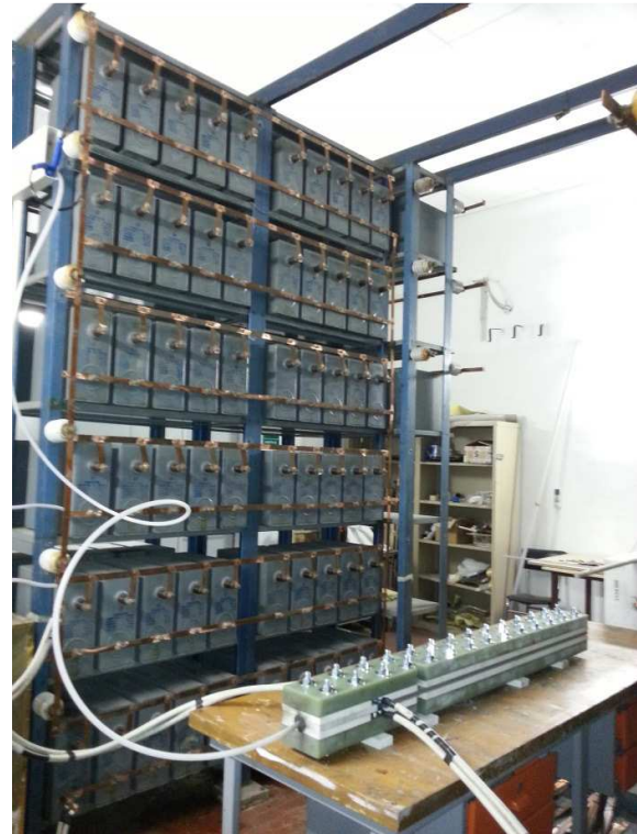
Figure 12. Bank of high voltage capacitors electrically connected to the railgun.
