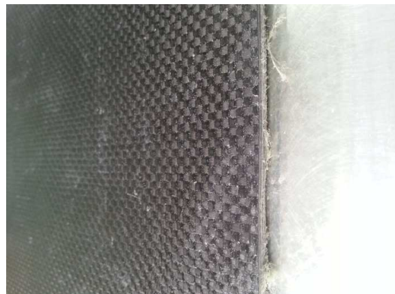
Figure 4. First kind of layered material. First layered CFRP+Kevlar structure after mechanical machining.
