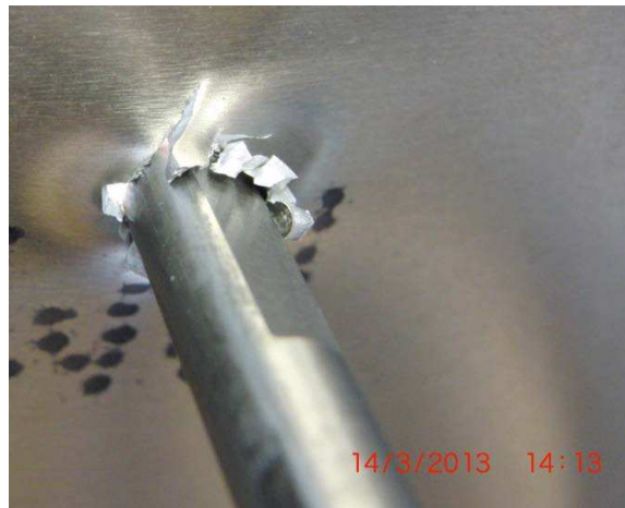
Figure 12. Penetration of 2mm thick Al 2024 plate
