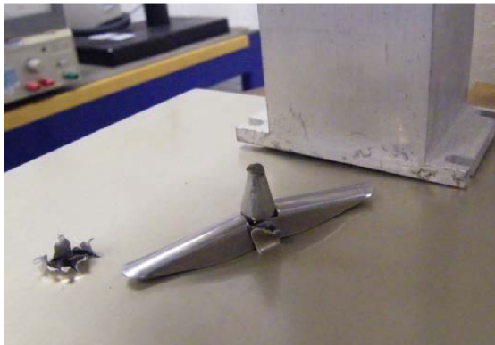
Figure 8. Successful barb deployment, note the second impact hole nearby showing the peeling nature of the panel skin failure
