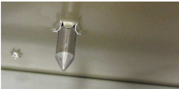
Figure 10. Penetration of Al/Al honeycomb (note barbs removed to show panel failure mode)
