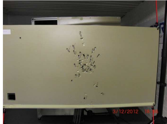
Figure 14. Lightweight single panel suspended with elastomer cord and penetrated multiple times at 10m
