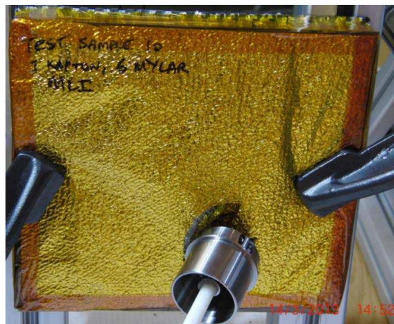
Figure 13. Penetration of CFRP/Al honeycomb with MLI on the outer face
