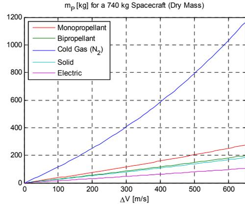
Figure 2. Fuel mass over  $\Delta v$  for different technologies
