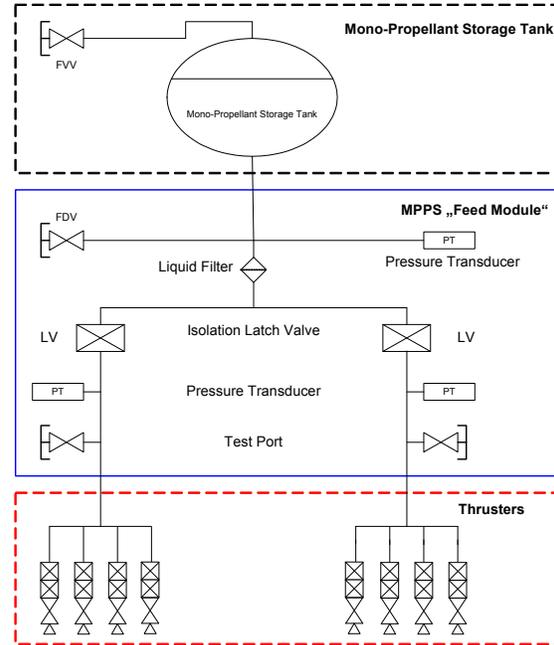
Figure 7. Jason-CS Propulsion Module Schematics
