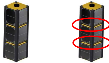
Figure 1. On the left is shown a CubeSat satellite from GomSpace. On the right is illustrated a similar satellite system fitted with two SDSS modules – in total 4 sails.
