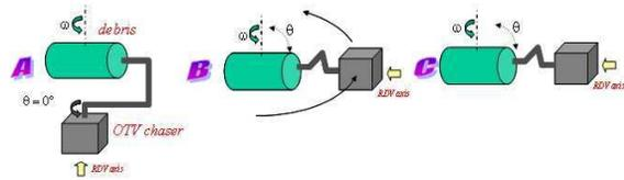
Figure 7: Options for capture and control of a debris with a robotic arm (MDA)
