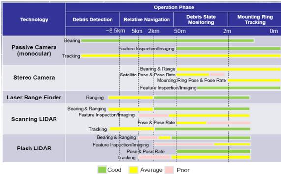
Figure 6: Typical technologies usable for short-range rendezvous between Chaser and debris (MDA)
