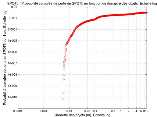
Figure 1: Cumulated probability of loss of Spot 5 function of the size of impacting debris (CNES)
