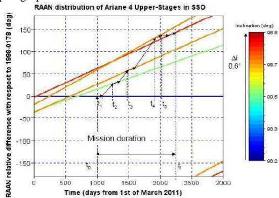
Figure 4: Typical use of RAAN drift during a multi-Target mission (CNES)
