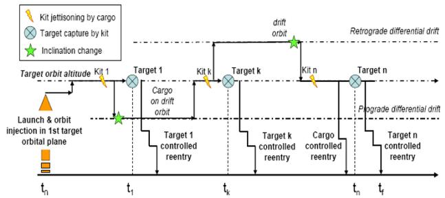
Figure 5: Schematic of a multi-Target mission using RAAN drift (CNES)
