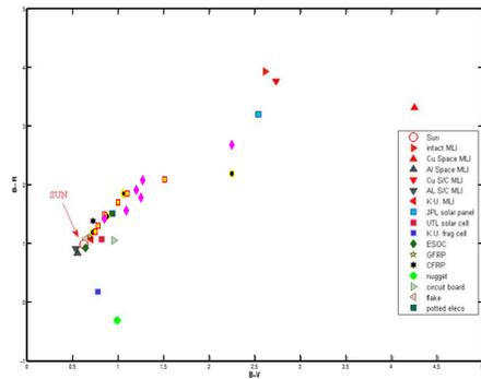
Figure 3. Photometric B-R vs. B-V color indices of our target superimposed to the Figure 1 of [1]
