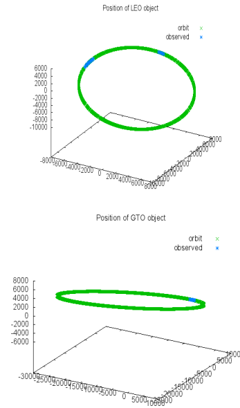
Figure 4: Representation of LEO and GTO orbits and the observation arc with a radar
