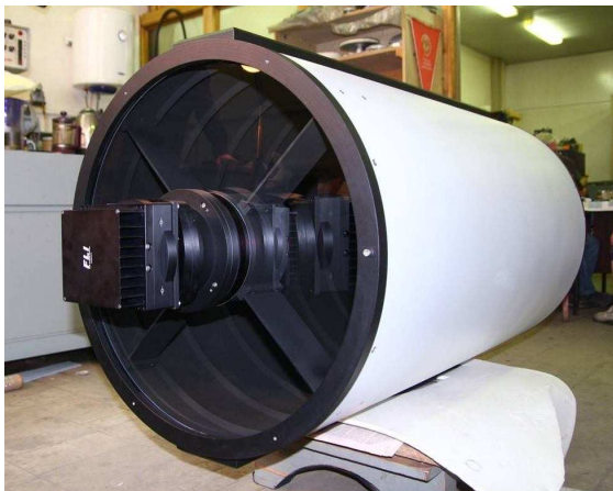
Figure 2. 65-cm SANTEL-650 telescope of new series.
