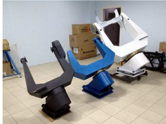
Figure 3. WS-240, WS-300, WS-500 folk mounts.
