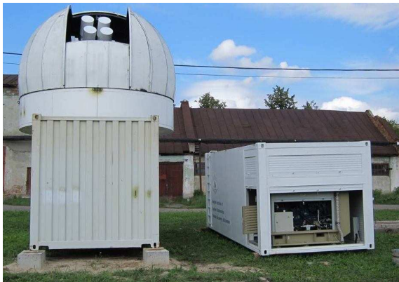
Figure 13. 4x19.2 cm telescope in dome and observer pavilion of EOP-2 observatory.
