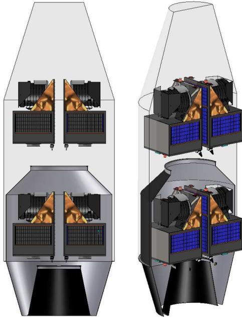
Figure 8: SBSS constellation in one VEGA launcher with adapted VESPA adapter
