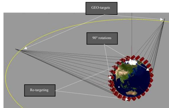
Figure 5: S/C attitude over one orbit, with GEO targets at 38.5° sun illumination
