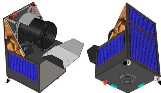
Figure 6: SBSS platform with telescope (external view)
