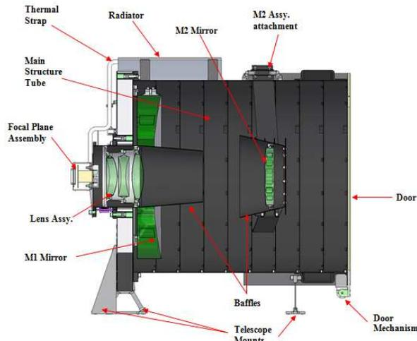
Figure 4: Cross section through the payload
