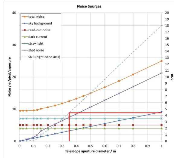
Figure 3: SNR and noise sources versus telescope aperture. The bold red line shows the SNR at an aperture of 350 mm.
