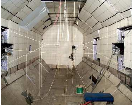
Figure 8. Inside view (down range) of the Range G target chamber. The interior wall of the range tank is covered with low density foam panels.
