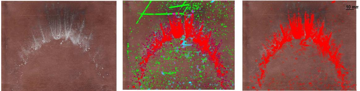
Figure 3. Witness plate analysis for shot no. 8656 (2.3 mm projectile at 5.34 km/s on a 10 mm Al6082-T6 plate, 45° impact): raw image (left), damage features recognized by the analysis (center), craters identified after “false positives” subtraction (right).
