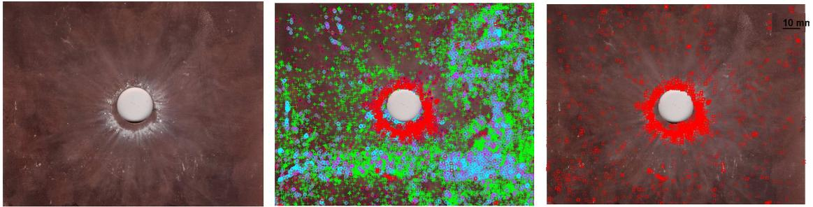
Figure 2. Witness plate analysis for shot no. 8646 (1.5 mm projectile at 5.20 km/s on a 10 mm Al6082-T6 plate, normal impact): raw image (left), damage features recognized by the analysis (center), craters identified after “false positives” subtraction (right).
