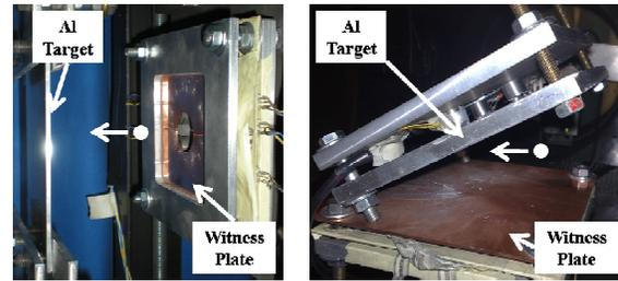
Figure 1. Target holder: normal (left) and oblique (right) impact configuration. In the normal impact configuration, a central hole is evident in the witness plate to allow the projectile pass through the plate and reach the target.
