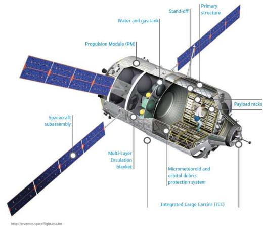
Figure 6. Automated Transfer Vehicle (illustration courtesy European Space Agency, ESA).
