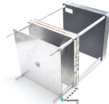
Figure 4. Example aluminum sandwich panel target (no. 2.3, experiment 5387) before impact testing.
