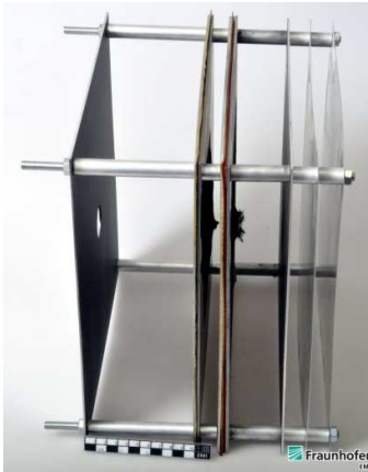
Figure 3. Example MLI target (no. 1.6, experiment 5397) after impact testing.
