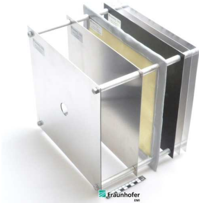
Figure 6. Example intermediate layer or reinforced box wall target (no. 5.2, experiment 5392) before impact testing.
