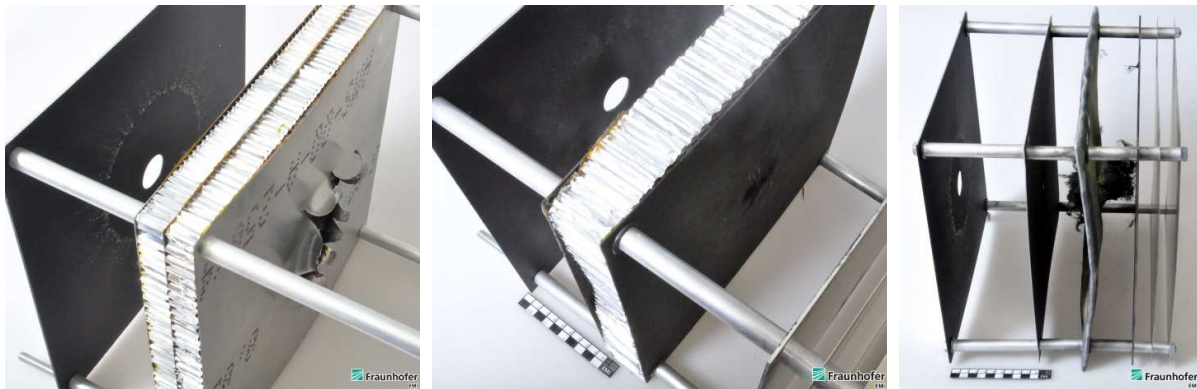
Figure 7. Example targets after impact testing. From left to right: aluminum sandwich panel (Target 2.3, experiment 5387), CFRP sandwich panel (Target 3.2, experiment 5404), intermediate layer or reinforced box wall (Target 5.2, experiment 5392).
