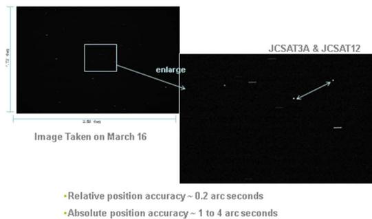
Figure 10, showing the improvement to the uncertainties when using relative angles for orbit determination
