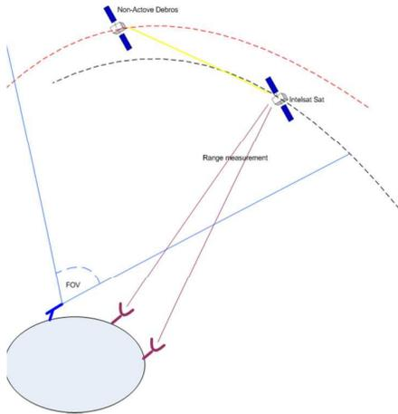
Figure 9, describing the concept of computing the orbit of the non-active object using relative angles from the active satellite which is also tracked with two station ranging.
