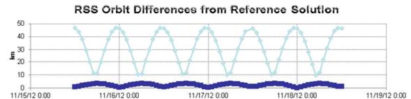
Figure 6, IS19 RSS orbit differences from reference two station ranging solution over 3 day span
