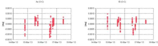
Figure 4, JSAT 5A optical measurement residuals from reference solution using two station ranging.
