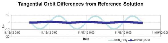
Figure 7, IS19 Tangential orbit differences from reference two station ranging solution over 3 day span
