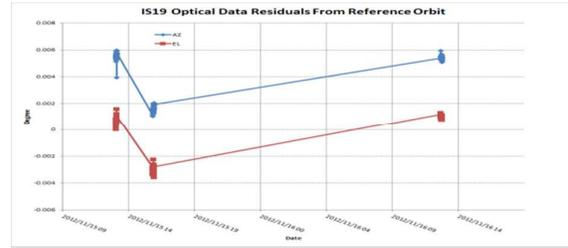
Figure 3, Data residuals for IS19 based on reference solution using 2 station ranging data.
