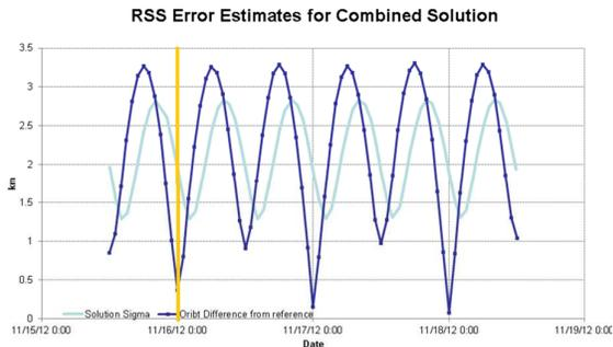
Figure 8, comparing the orbit differences with the predicted orbit error.
