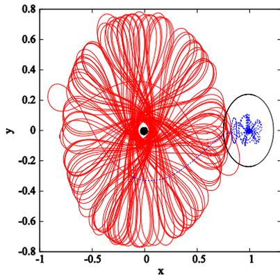
Figure 12.  $x$ - $y$  projection of a weak capture trajectory (blue) at the Moon obtained by propagating the unstable invariant manifold of a halo  $L_1$  orbit and endgame strategy (red). Synodical reference system with non-dimensional units. The black circle represents the Hill's sphere at the Moon.
