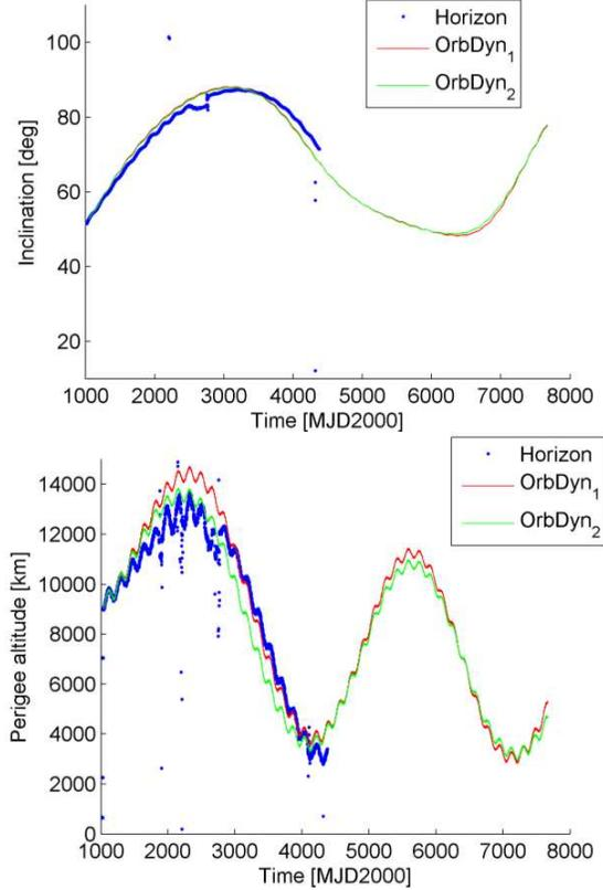
Figure 1. Orbit evolution of INTEGRAL between 2002 and 2021. Blue line: ephemerides (Horizon, NASA), red and green: numerical propagation with  $J_2$  and luni-solar effect with Cook [1] and Chao's formulation [6].
