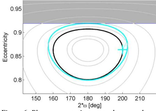
Figure 6. Phase space trajectory to decrease the perigee to 600 km. The cross indicates where the  $\Delta v$  manoeuvre is applied. From the top:  $M_1$ ,  $M_2$ ,  $M_3$ ,  $M_4$ .
