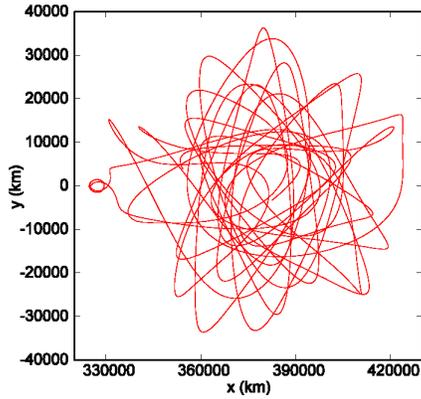
Figure 10. Example of weak capture trajectory at the Moon.  $x$ - $y$  projection in the synodical reference system, where the Moon is located at (379729.32, 0) km.
