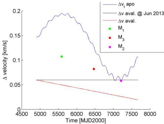
Figure 9.  $\Delta v$  requirements to decrease the perigee with a single manoeuvre at the apogee.
