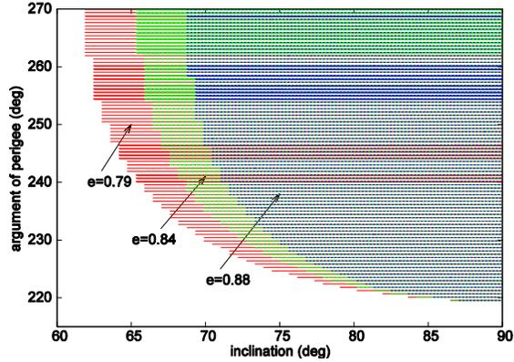
Figure 2. Range of inclination and argument of perigee (in the Earth-Moon orbital plane) for different values of the eccentricity, associated with a decrease of the argument of the perigee.
