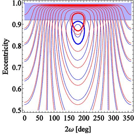
Figure 5.  $(2\omega, e)$  phase space evolution under third-body perturbation. Blue lines:  $\Theta = 0.03804$ , red lines:  $\Theta = 0.01513$  which corresponds to an increase of eccentricity of 0.1 with respect to INTEGRAL's.
