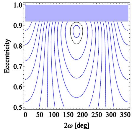
Figure 3  $(2\omega, e)$  phase space evolution under third-body perturbation. Black line: INTEGRAL-like s/c.
