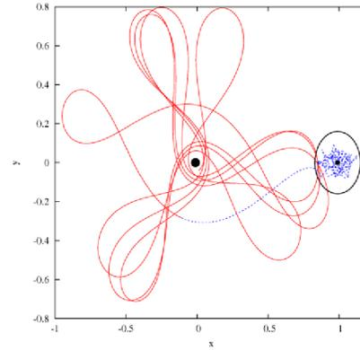
Figure 11.  $x$ - $y$  projection of a weak capture trajectory (blue) at the Moon obtained by propagating the unstable invariant manifold of a vertical Lyapunov  $L_1$  orbit and endgame strategy (red). Synodical reference system with non-dimensional units. The black circle represents the Hill's sphere at the Moon.
