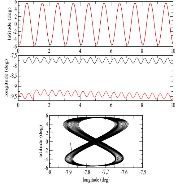
Figure 3. Time series of latitude and longitude for the Telecom-2D satellite (top) ; the X-axis is time (number of days from 8th August 2012, and covering a period w/o any maneuver). The third plot is the ground track trajectory. Black curves correspond to the reference orbit (computed with the Romance CNES s/w), the red ones to the trajectories obtained with our approach.
