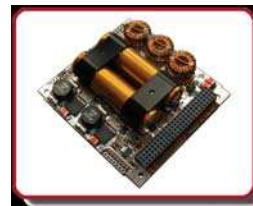
Figure 6. Nanosatellite power and energy storage module (Courtesy of ISIS Cubesat Solutions)
