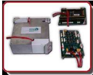
Figure 3. Nanosatellite propulsion and attitude control module (Courtesy of ISIS Cubesat Solutions)
