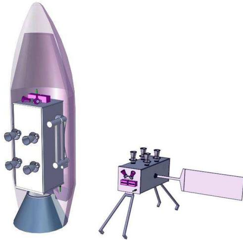
Figure 16. Clamping mechanisms option system design shown in stowed configuration (left) and de ployed configuration (right). This configuration shows the optional robotic arm on the right panel in the stowed configuration
