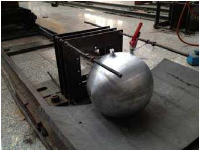
Figure 2. Spherical Gas-filled Pressure Vessel Used in the Tests
