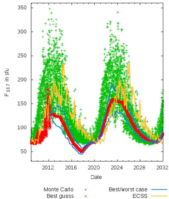
Figure 2. Example for an OSCAR solar activity forecast in solar cycle no. 24 for the different modeling approaches.
