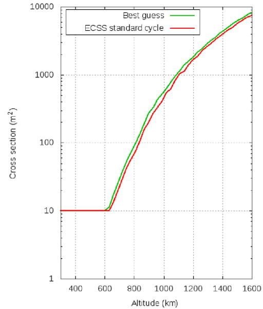
Figure 3. Required cross-section for a drag augmentation system in order to be compliant with the SDMG, for a spacecraft in an initially circular near-polar orbit with a cross-section of  $10 \text{ m}^2$  mass of 1,000 kg and drag coefficient  $C_D = 2.2$ . Results for two solar and geomagnetic activity scenarios are shown.
