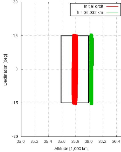
Figure 5. The orbital evolution within 100 years for the initial orbit as well as the recommended altitude given via Equation 3.
