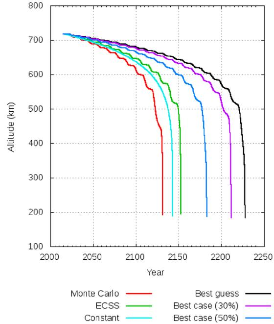
Figure 4. Orbital lifetime of Cryosat-2 for an initial orbit of  $710 \times 726$  km, 92 deg inclination, starting in 2015/01/01. The cross-section was assumed to be  $3.4 m^2$ . Different scenarios for solar and geomagnetic activity were applied.
