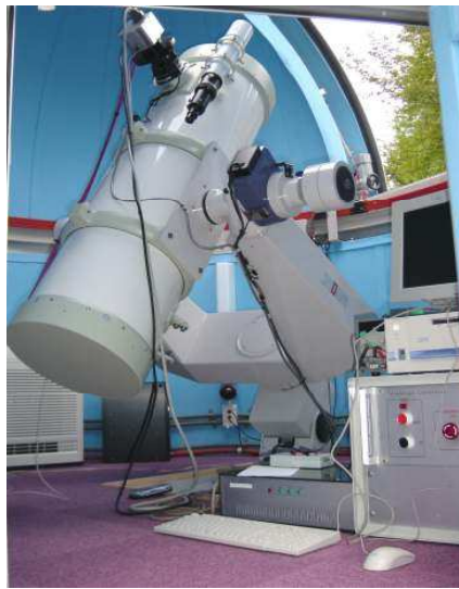
Fig.2(b). Fork-type mount and 35cm telescope
