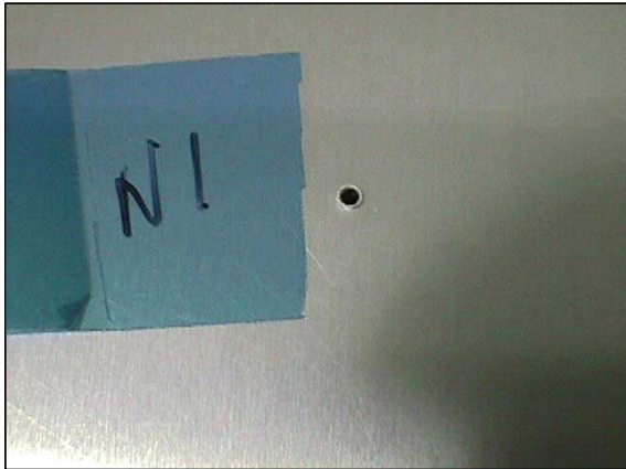
Figure 11. Hole found in the space debris shield after the first flight of the MPLM to the ISS in 2001
