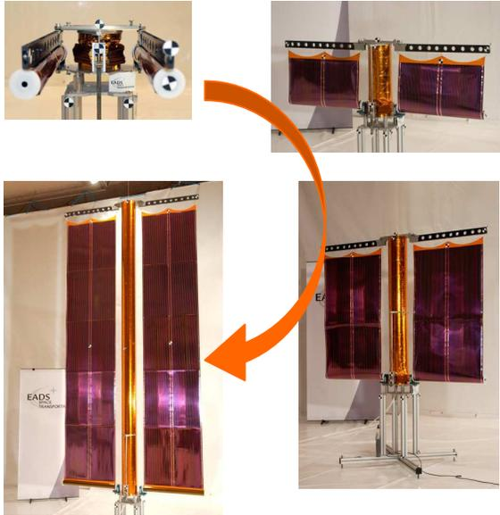
Figure.3 : Gossamer structure deployment concept
