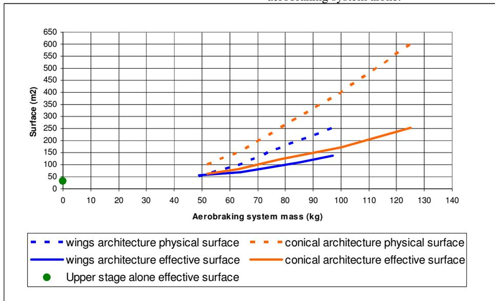
Figure 7 : effective and physical surfaces function of aerobraking system mass for both architectures
