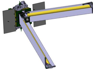
Figure 1 : IDEAS system deployed on Microscope satellite
