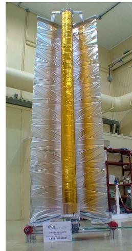
Figure 2 : aerobraking system wing - 3 metres breadboard
