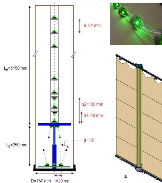
Figure 11 : In-orbit polymerisation technology overview
