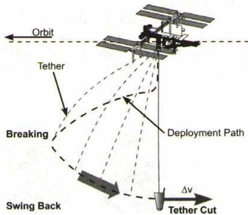
Figure 13: Principle of a momentum exchange tether [4].
