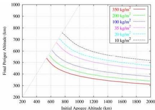
**Figure 10:** Required perigee lowering to achieve a remaining orbital lifetime of less than 25 years for an object with a given mass-to-area ratio, and for an initially circular orbit [6]. The no-maneuver results are depicted along the dotted line for circular disposal orbits.
