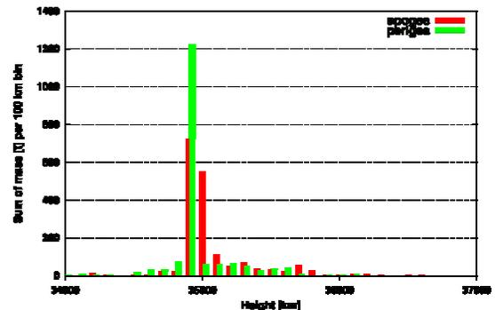
Figure 6: Distribution of the mass of on-orbit objects in the GEO regime (tons per 100 km altitude bin).
