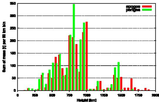
Figure 4: Distribution of the mass of on-orbit objects in the LEO regime (tons per 50 km altitude bin).
