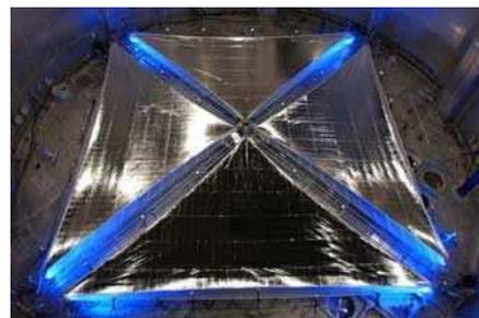
**Figure 12:** Concept of a  $20\text{m} \times 20\text{m}$  deployable solar sail (courtesy NASA).
