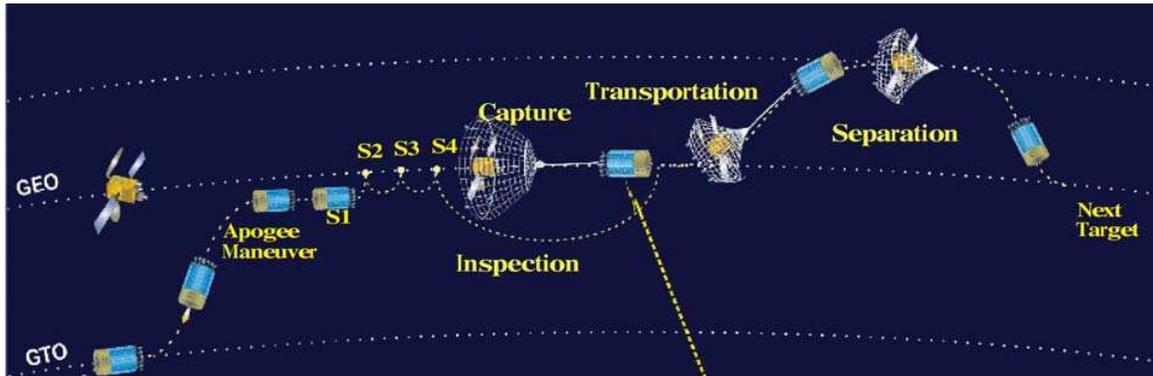
**Figure 15:** Concept of a remover satellite for tugging GEO objects to a GEO disposal orbit (courtesy EADS Astrium).
