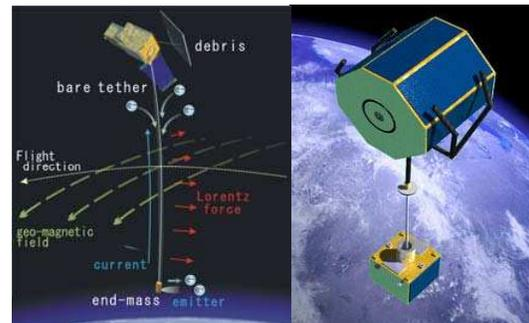
Figure 14: Principle of a conductive tether and its application for de-orbiting (courtesy JAXA).
