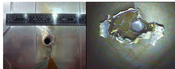
Figure 4. MMOD impacts on STS-118 LH4 radiator.
