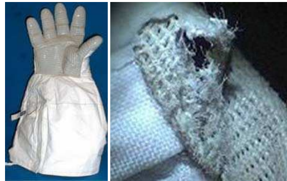
Figure 1. Damage to crewmember Curbeam's Phase IV glove following EVA 3 of STS-116
