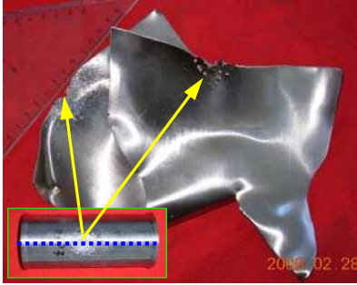
Figure 7. Crack Growth of Rupturing Vessel
