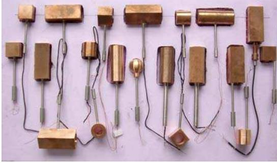
Figure 2. Photo of all solid copper heat transfer models
