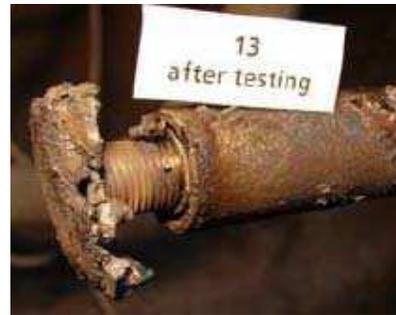
Figure 21. TI/CFRP model after 220 s test time
