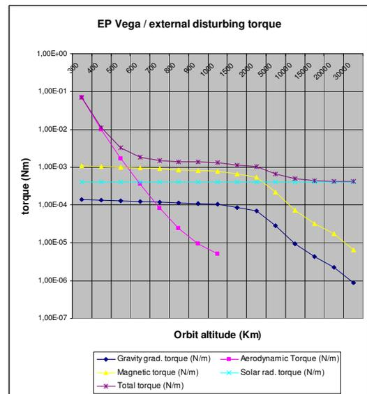
Fig 6: Environmental torques / Forces vs altitude
