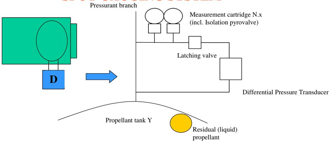
Fig 11: Spot Gauging System schematic
