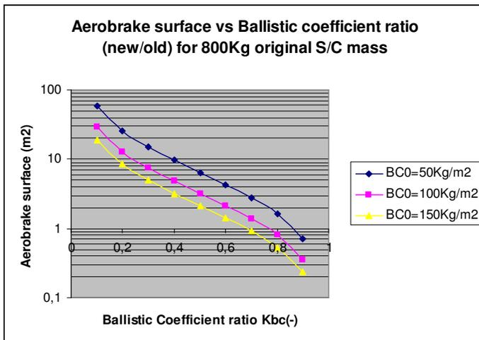
Fig 5: Ex. of calc diagram for the aero-brake surf. of a 800 Kg S/C
