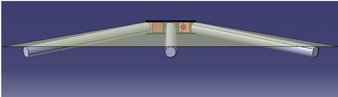
Fig 9a: detail of the aero-braking (deployed) shield
