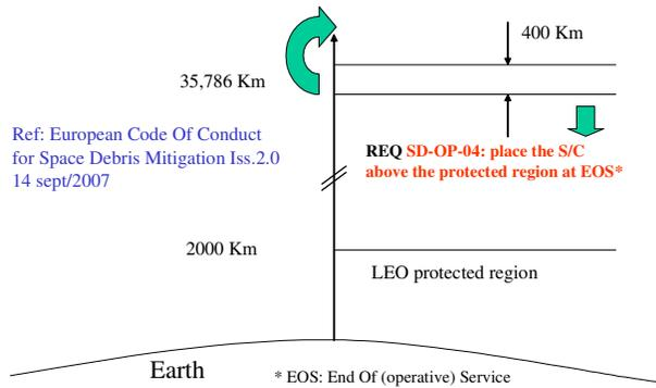
Fig 7: Requirement for GEO protected altitude range
