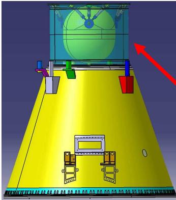
Fig 10a: Detail of the CAOS propellant tank
