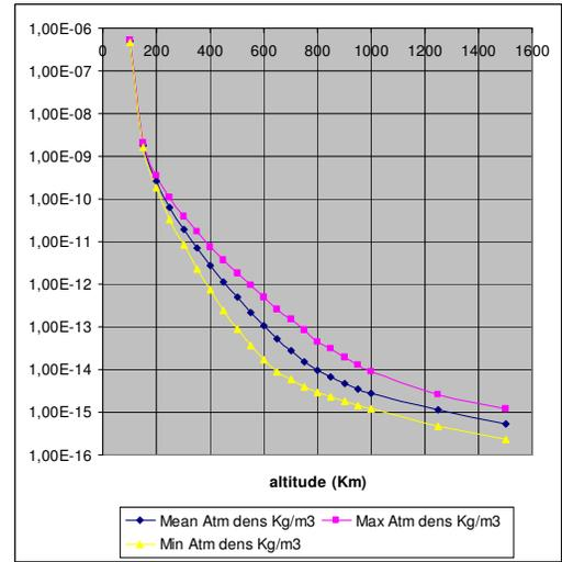
Fig.4: Equiv atmospheric densities vs altitude
