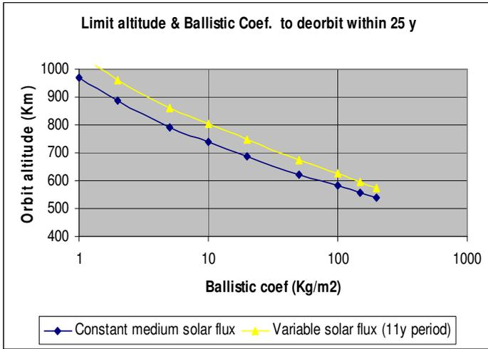
Fig 3: Limit altitude & ballistic coeff for 25y re-entry time
