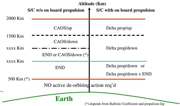
Fig 8: trade.off diagram for de/re-orbiting approach from LEO
