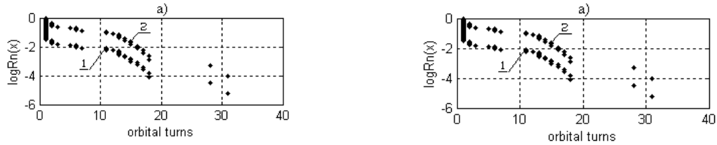
Figure 9. The logarithmic graphs of empirical function of reliability according to the sensor CS-4
