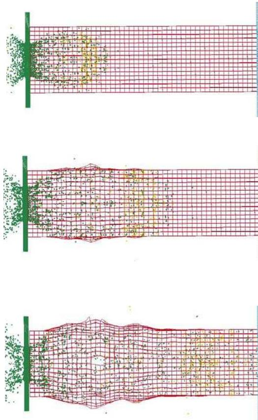
Figure4. Debris cloud in single cell (HC-2)
