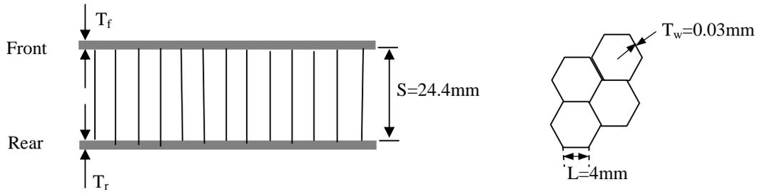
Figure2. The simulated honeycomb configuration
