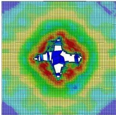
Figure9. Rear face damage in HC-2
