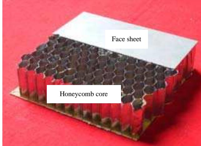
Figure1. Structure of honeycomb sandwich panel
