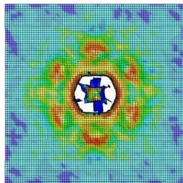
Figure11. Rear face damage in HC-4
