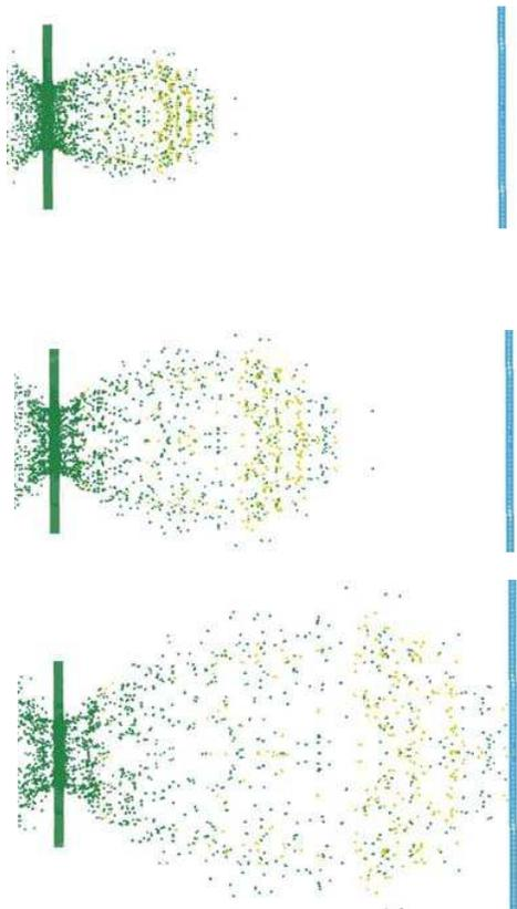
Figure3. Debris cloud in Whipple Shield (HC-1)
