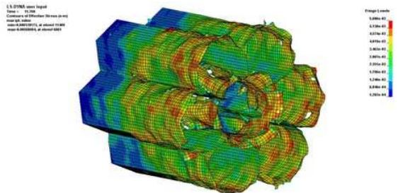
Figure6. Damage of honeycomb cores in HC-4
