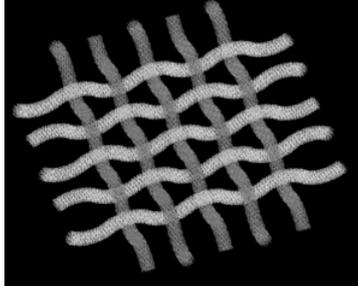
Fig 3. SPH particle model of AL mesh
