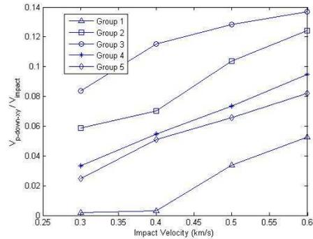
Fig 9. tangential velocity of downrange fragments from projectile vs impact velocity
