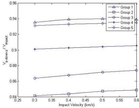
Fig 7. Axial velocity of downrange fragments from projectile vs impact velocity
