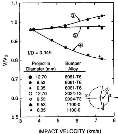
Fig 8. Debris cloud axial velocity vs impact velocity<sup>[8]</sup>
