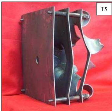
Figure 4. Damage of multi-plate
