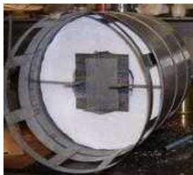
Figure 2. The rear view of a collector with an attached aluminium plate target
