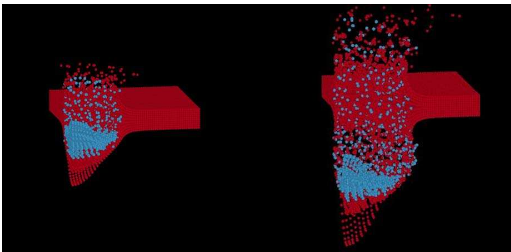
Figure 5. Cylindrical projectile with impact velocity 7 km/s at 1 \mu s (left) and 2 \mu s (right) after impact
