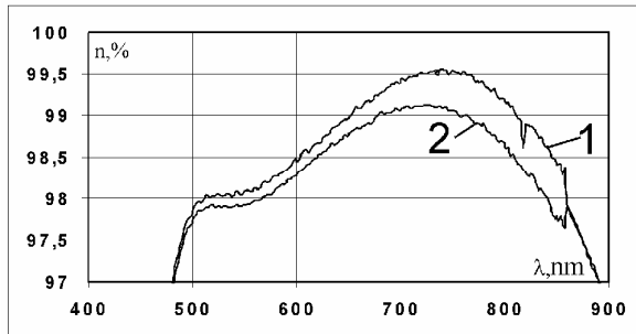
Figure 7 - Dependence of optical glass transmission on the wavelength
