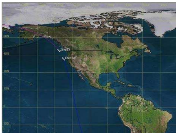
Figure 11: Groundtracks extracted from visualfocus for the ENVISAT vs. ZENITH-2 conjunction event
