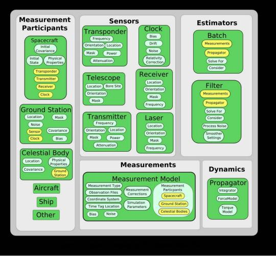
The sensor models contained in GMAT include but are not limited to clocks, receivers, transmitters, transponders and lasers. The user can create and configure sensors for their application and attach the sensor to the appropriate parent object such as a spacecraft or ground station.
