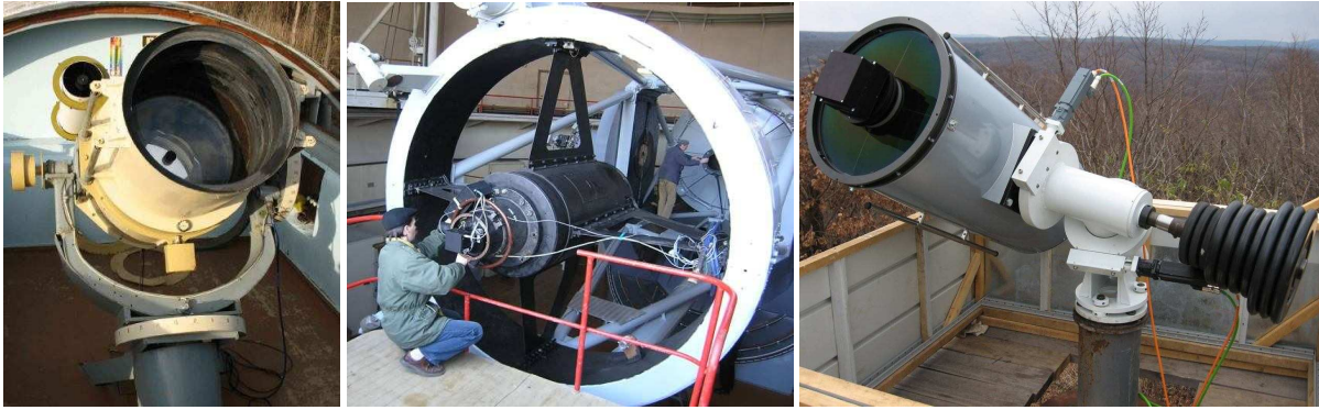
Figure 3. Examples of telescopes for the faint fragment observations: 64-cm AT-64 and 2.6-m ZTSh in Nauchniy-1, new 50-cm VT-40/500 in Ussuriysk.
