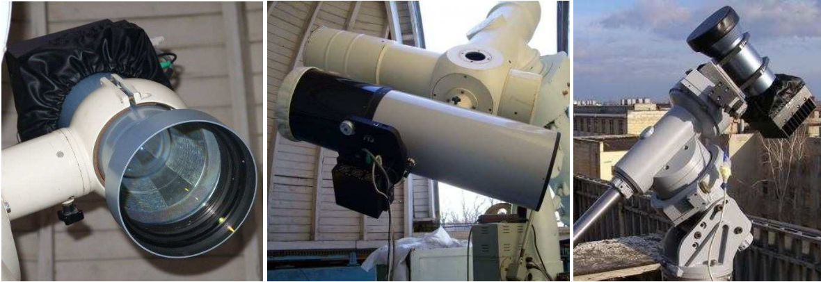
Figure 5. Examples of telescopes for observations of the HEO and LEO objects: - 12.5-cm VT-15e and 25-cm GAS-250 in Ussuryk and 12.5-cm VT-15e in Tiraspol
