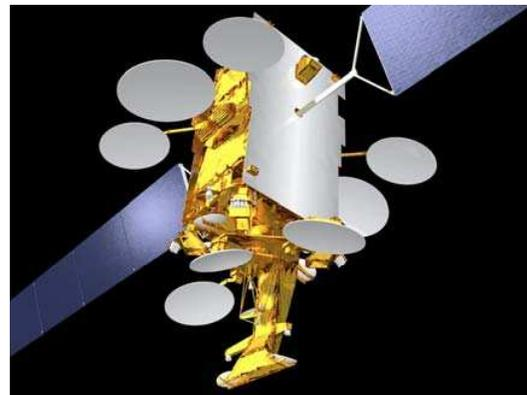
Figure 3. Sketch of a modern large GEO telecommunication satellite showing the main exposed surfaces
