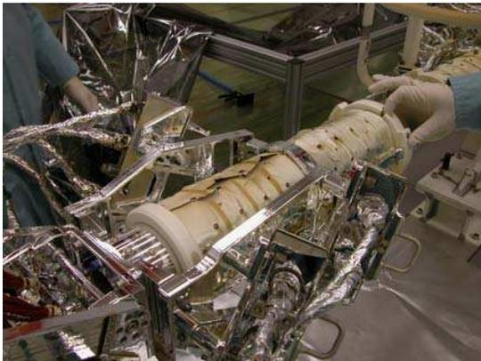
Figure 1. Damaged MLI on HST solar array drive after retrieval
