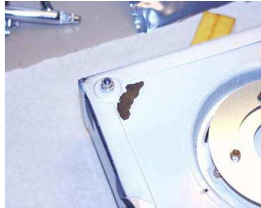
Figure 2. Damaged metal coating on antenna following thermal tests
