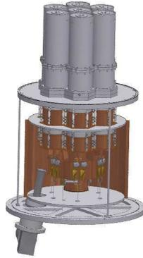
Figure 2. CAD model of the Effelsberg multi-beam receiver
